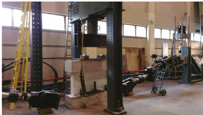
(b) Photo of shear wall inside the actuator
