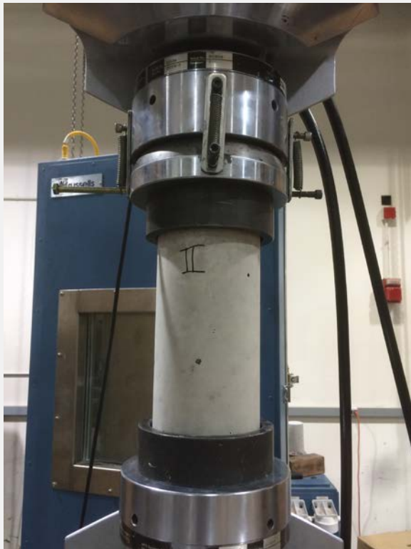
Compression testing according to ASTM C39
