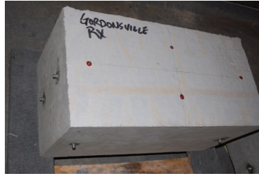
Figure D.18: Concrete expansion block tested by Prof. E. Giannini
