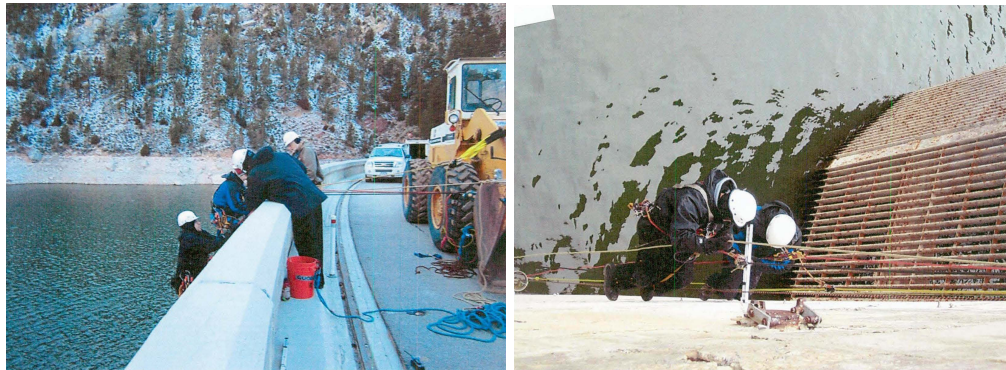
Figure A.5: Climb Team members measuring upstream dam face to plumb line (lung2012)
