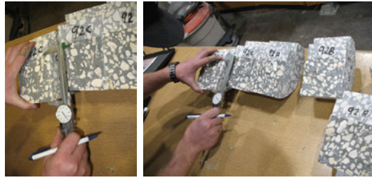
Figure A.8: Measuring specimen dimensions
