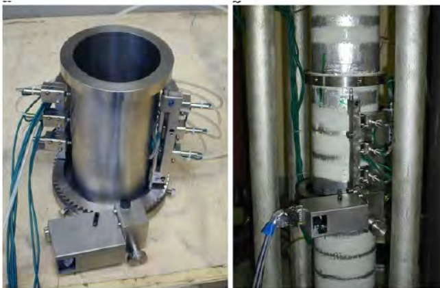
Figure 3.156: Characteristics of the 48 specimens including the steel rings and strain measurements by an automated device; Multon and Toutlemonde (2006)
