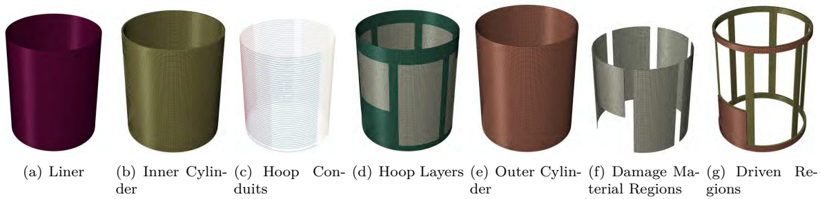
Figure 8: Group 7 Finite element analyses; global sub-model (ADAMS Accession No. ML 102861026, 2010)
