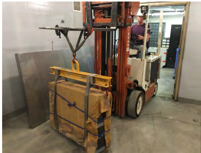
Figure 3.16: Placing shear specimen in fog room with forklift
