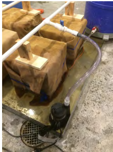
Figure 3.18: Sump pumps used to power sprinkler system
