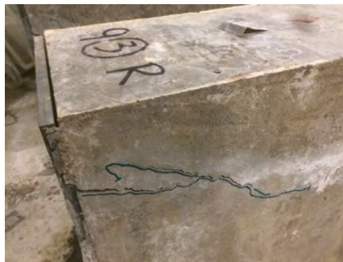
Figure 8.4: Cracking in Shear Specimens
