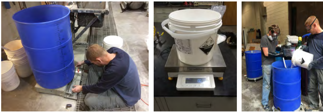
Figure 3.20: Weighing water and NaOH for NaOH solution preparation and mixing NaOH Solution
