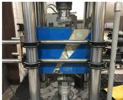
(b) Shear test with axial confinement (missing in FSEL tests)
