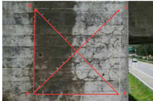
Figure 2.6: Determination of the crack-index along the lines A-B, A-C, A-D and B-C. Side of the square = 1 m, Leemann and Griffa (2013)
