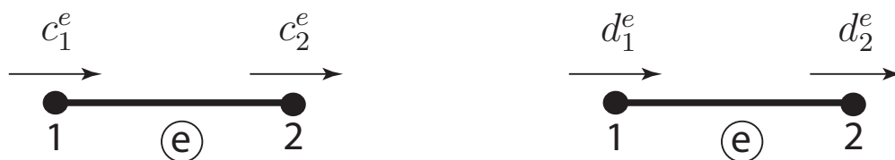
Figure 2.12. Nodal values of weighting function c_a^e and displacement d_a^e , local node a = 1, 2 .
