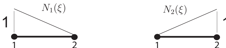
Figure 2.11. Linear shape functions for 2-noded element in natural coordinate \xi . N_1 = (1 - \xi)/2 , N_2 = (1 + \xi)/2 .
