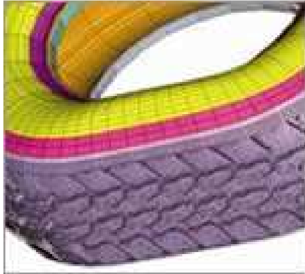
Figure 5.2. A car tire under constant angular velocity, and thus no rotation of deformed part with respect to reference frame (simulia.com).
