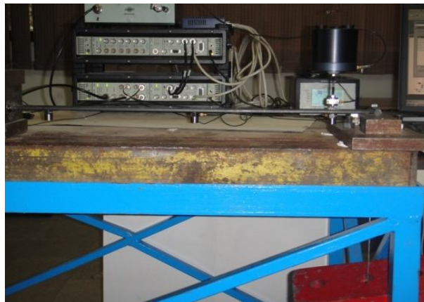
Figure 2: The test set-up of frictionally supported beam
