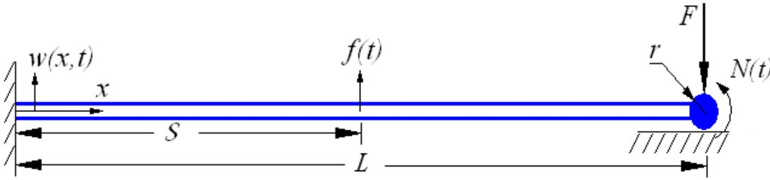
Figure 4. A slender beam with frictional contact boundary condition
