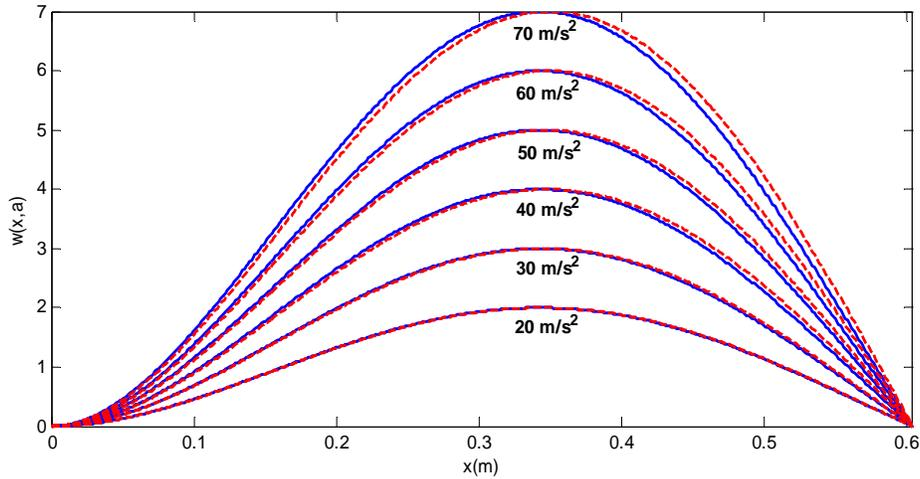
Figure 5. Comparing NNMs obtained by equivalent linearized system (red) and the first mode of the base linear system (blue)
