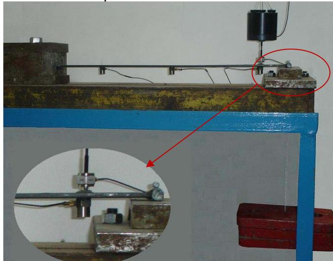
Figure 1. The test set-up of frictionally supported beam
