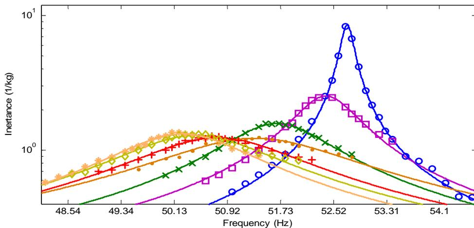
Figure 3. Measured and fitted frequency responses at response amplitudes of  $10 \text{ m/s}^2$  (circles),  $20 \text{ m/s}^2$  (squares),  $30 \text{ m/s}^2$  ( $\times$ ),  $40 \text{ m/s}^2$  (points),  $50 \text{ m/s}^2$  (+),  $60 \text{ m/s}^2$  (diamonds), and  $70 \text{ m/s}^2$  (\*).
