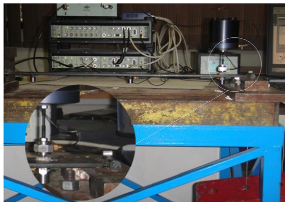
Fig. 2. The test set-up of frictionally supported beam.
