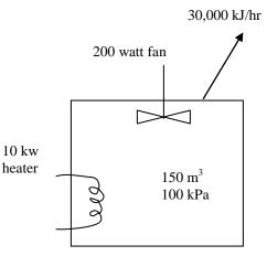
d) The homeowner is considering replacing the electric heater with a steam radiator. Steam enters the radiator at 200 kPa and 150  $^{\circ}$ C, and leaves as saturated liquid at the same pressure. What is the mass flow rate of steam required to keep the house at 22  $^{\circ}$ C from 5 PM to 8 AM?
