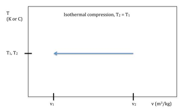
**PROCESS** from state 1 to state 2 is a compression. PATH is isothermal.
