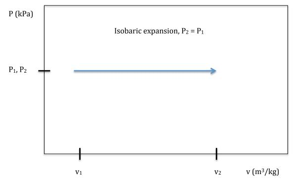
PROCESS from state 1 to state 2 is an expansion. PATH is isobaric
