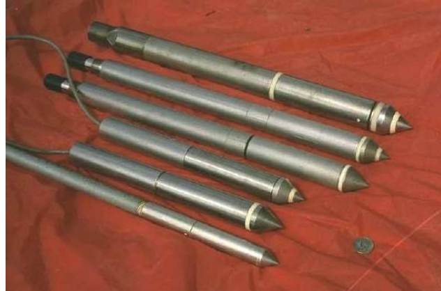
(a) image courtesy of Khalid Alshibli, (b) Cone penetrometers (see footnote* on previous page Louisiana State University. for image reference).
